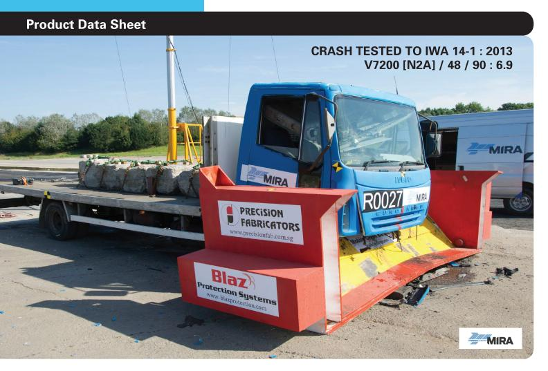
**MCB** // is a new generation of portable barrier system that is designed to meet the growing hostile vehicle threats.
